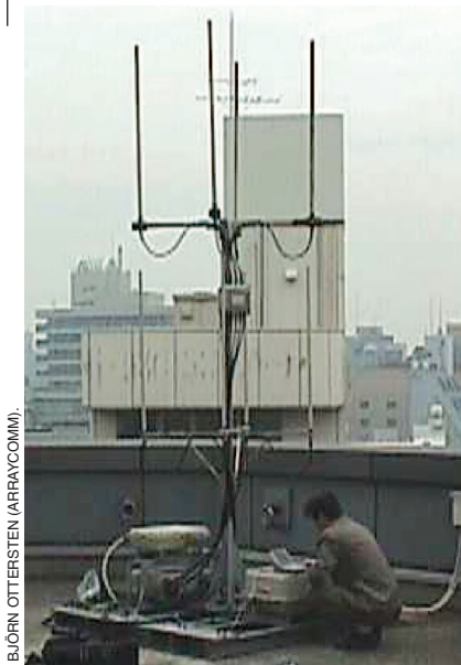
First SA base station of ArrayComm for cellular mobile communication networks (Asian PHS Standard), available since 1997.
